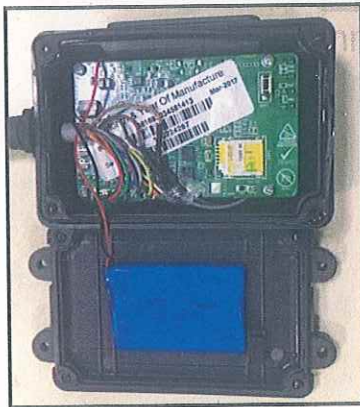
After Water Test
